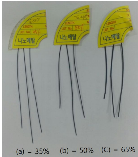
Fig. 4.1. Change in thickness of the Flexinol( \varnothing=500\mu\text{m} ) with the degree of cold-rolling; (a) 35, (b) 50 and (c) 65%.
