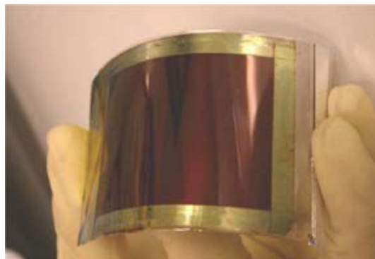
Fig. 16 Flexible DSSC with metal film
