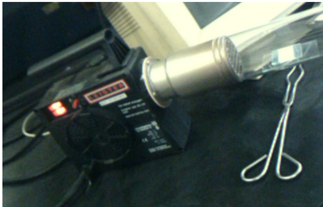
Fig. 22 Sintering of samples by a heater
