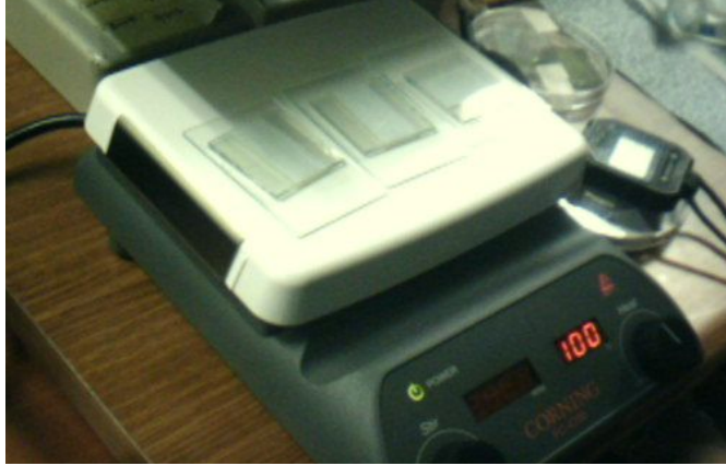
Fig. 21 Soft sintering of samples on a hot plate
