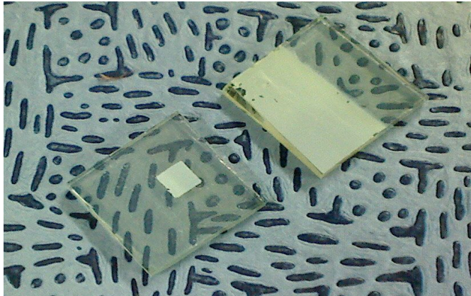
Fig. 23 Prepared working electrode
