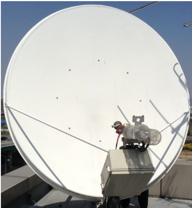
Figure 3(a): Parabolic antenna for 12.25 and 20.73 GHz receiving beacon signal.
