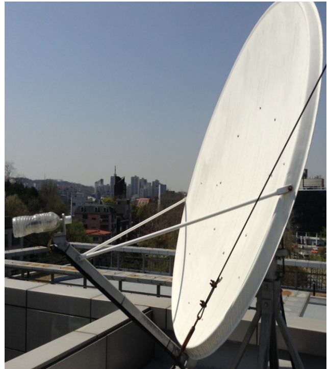
Figure 3(b): Parabolic antenna for 19.8 GHz receiving beacon signal.
