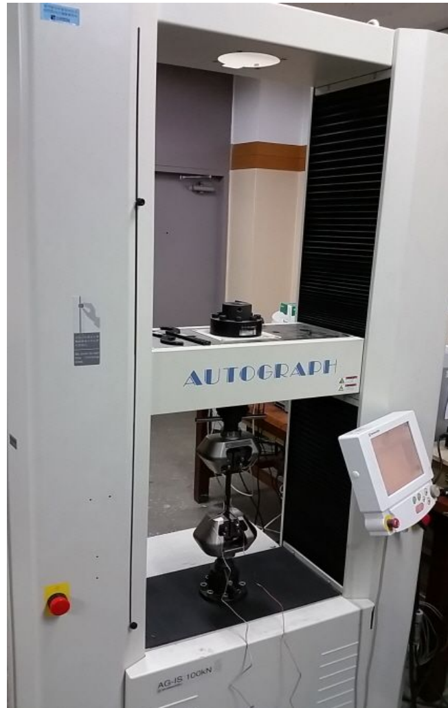
Photo 3 Universal testing machine
