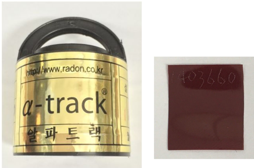
Figure 26. Radon cup (alpha track) and solid-state track detector (LR-115).
