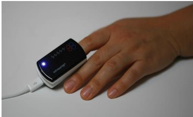
Fig. 3.2 Experimental device to measure PPG
