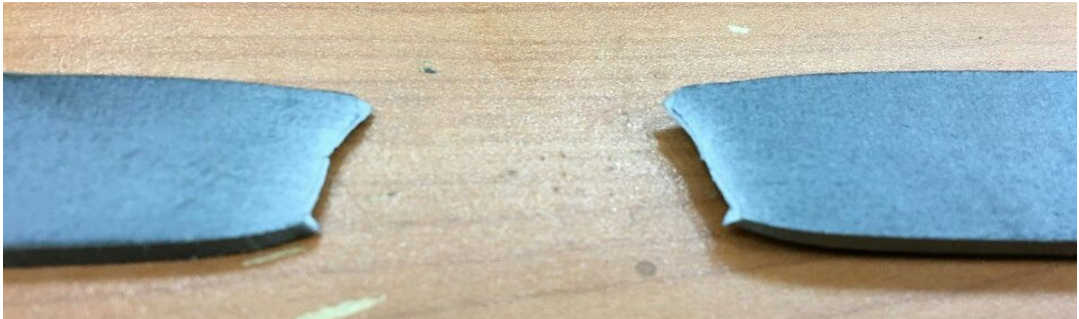
Fig. 4.4 Tensile fracture surface of SS400
