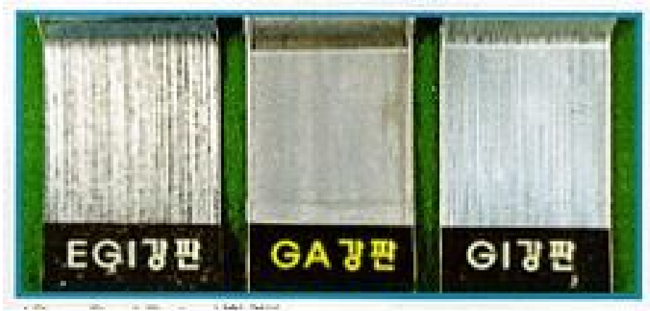
Fig. 1.1 Comparing EGI, GA and GI steel sheet
