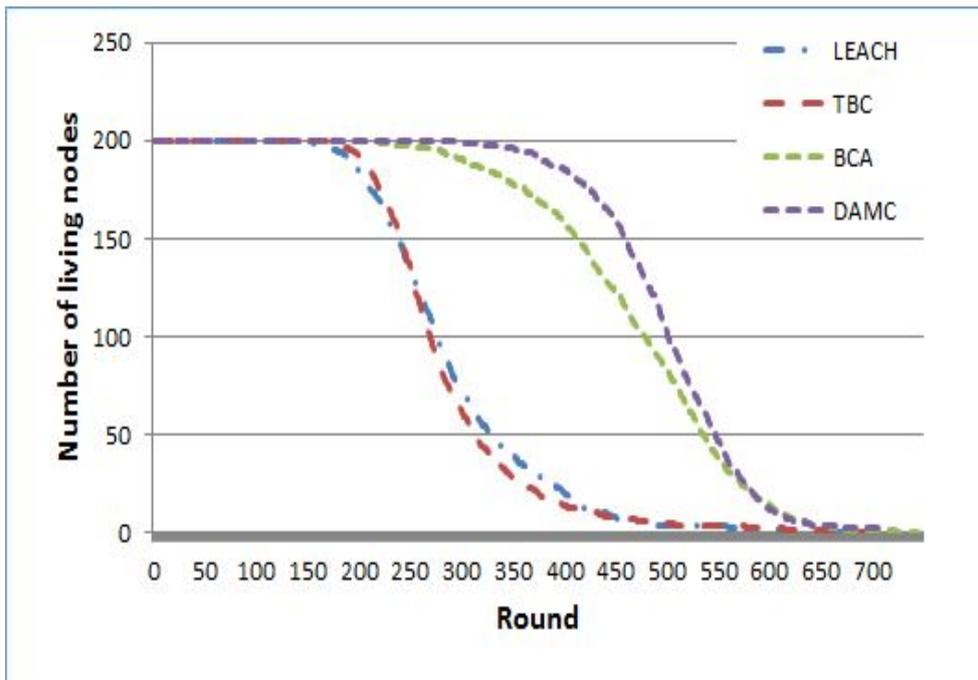
Figure 8. Network lifetime when 200 nodes are deployed according to the normal distribution with mean of (50, 50) and variance of ( $\pm 10$ ,  $\pm 10$ ).
