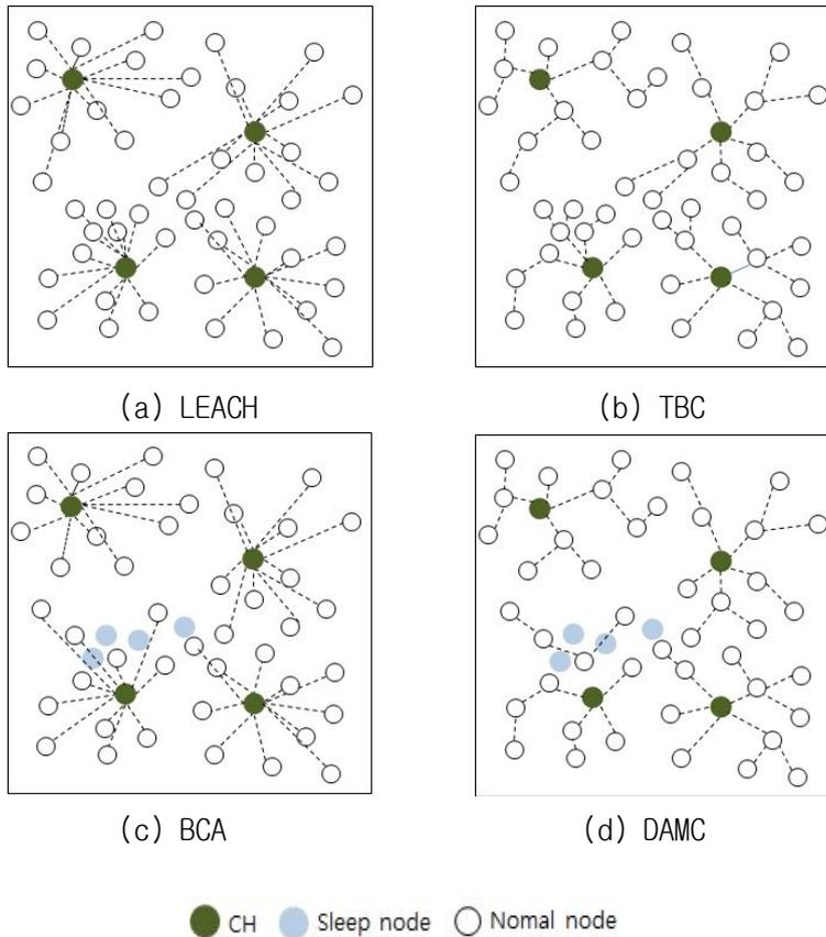
Figure 3. Examples of cluster formation in an irregularly deployed WSN
