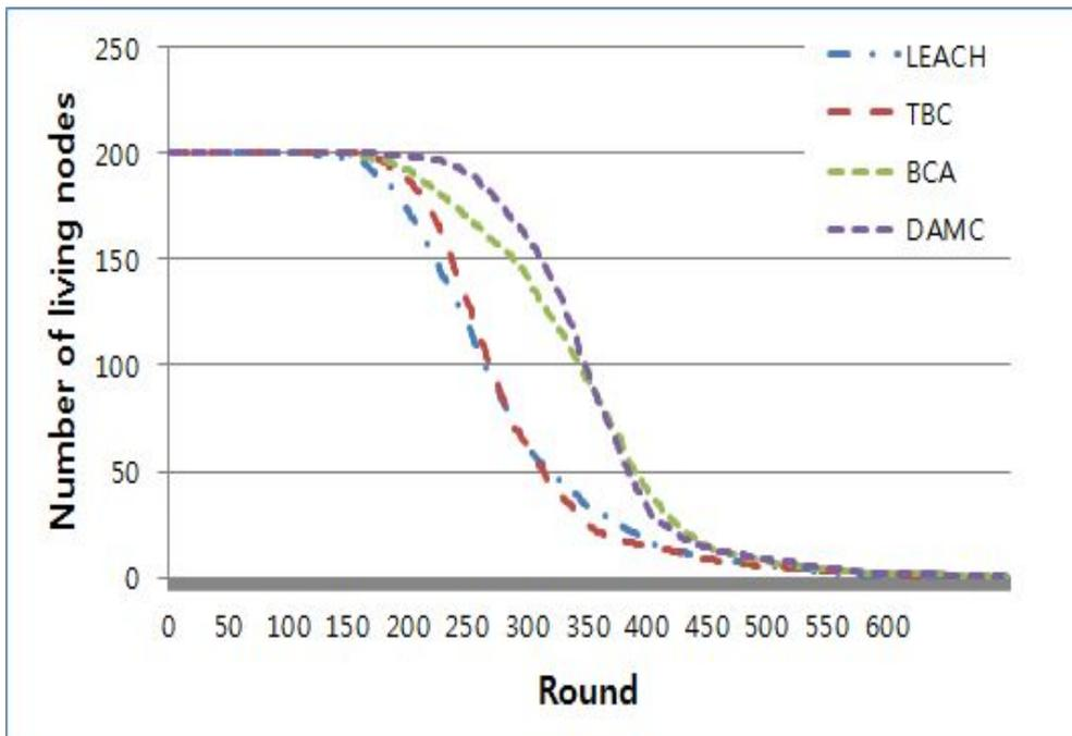
Figure 9. Network lifetime when 200 nodes are deployed according to the normal distribution with mean of (50, 50) and variance of ( $\pm 20$ ,  $\pm 20$ ).
