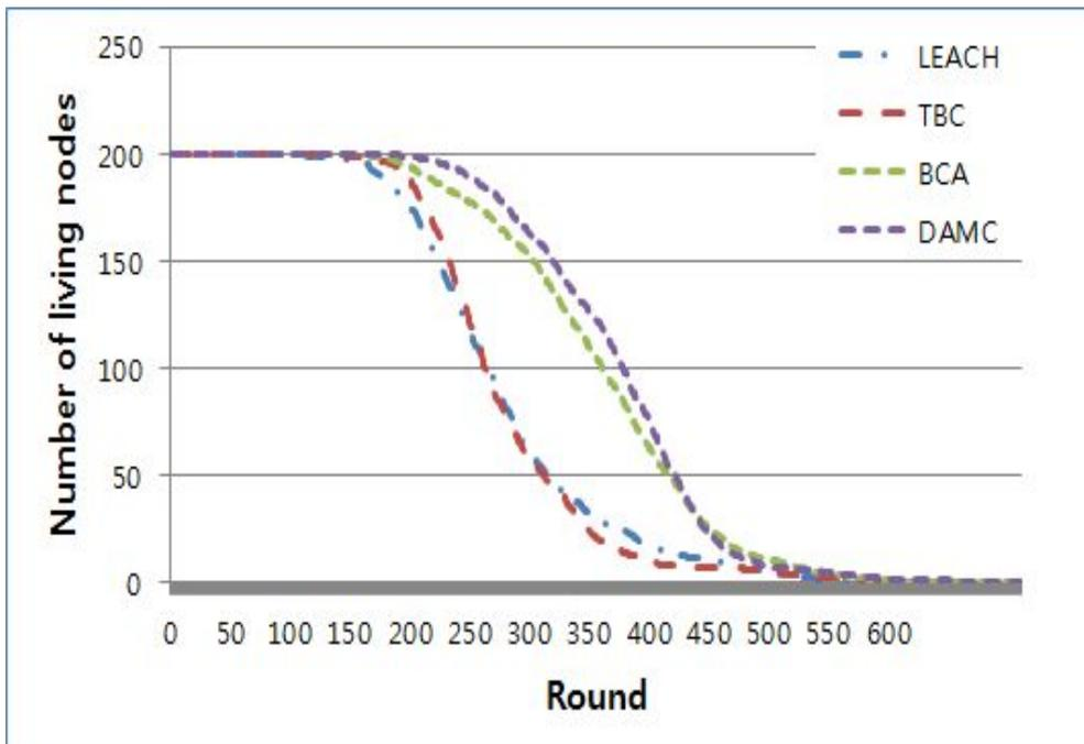
Figure 11. Network lifetime when 200 nodes are deployed according to the exponential distribution with mean of  $(50 \pm 20, 50 \pm 20)$ .
