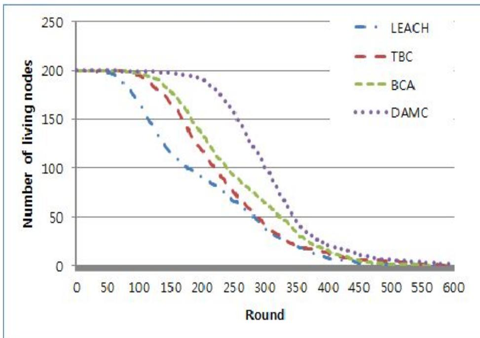
Figure 7. Network lifetime when 100 nodes are deployed in the region of  $25 \times 25 \text{ m}^2$  and the other 100 nodes are deployed in the other regions.
