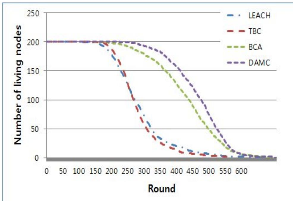
Figure 10. Network lifetime when 200 nodes are deployed according to the exponential distribution with mean of  $(50 \pm 10, 50 \pm 10)$ .
