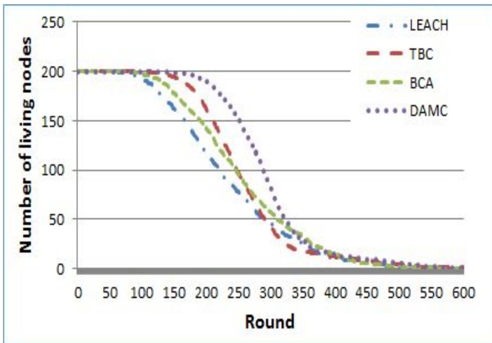
Figure 6. Network lifetime when 100 nodes are deployed in the region of  $50 \times 50 \text{ m}^2$  and the other 100 nodes are deployed in the other regions.
