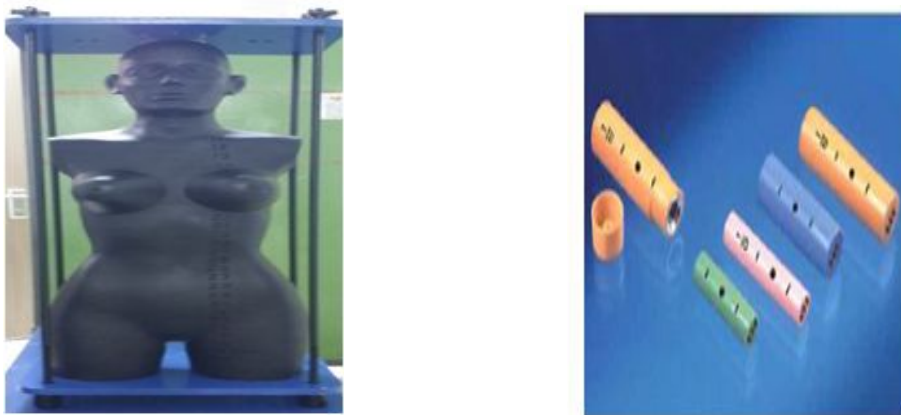
Figure 8. Rando Man Phantom & Glass dosimeter Element.
