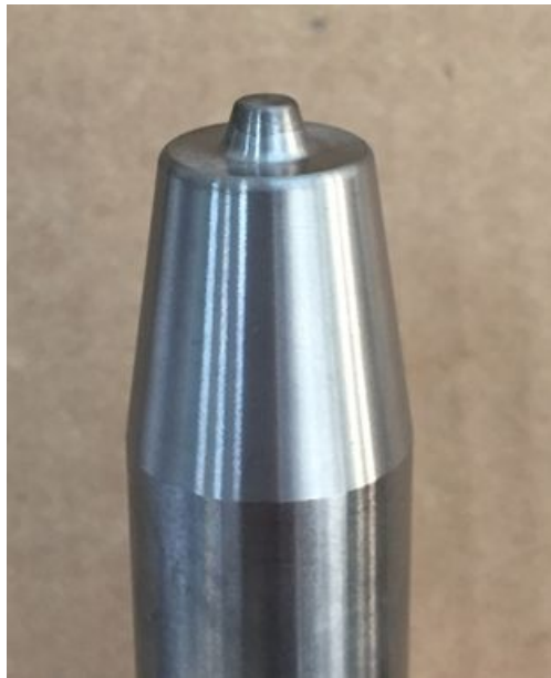
Fig. 2.2 Tool details used for FSJ
