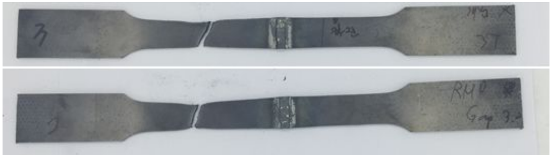
Fig. 4.11 Fractured specimen of RMD-GMAW after SS400 tensile test
