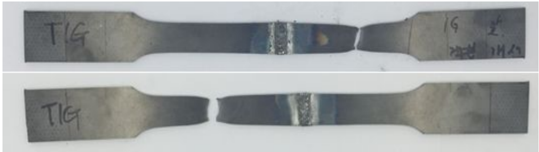
Fig. 4.10 Fractured specimen of GTAW after SS400 tensile test
