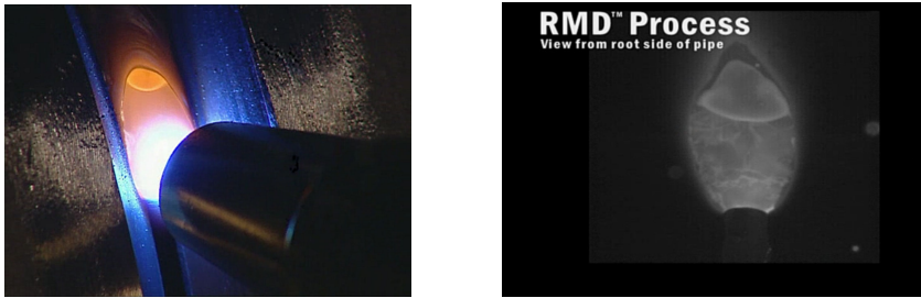
Fig. 5.2 Congiguration of RMD-GMAW Process
