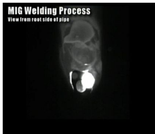
Fig. 2.15 Short Circuit Transfer
