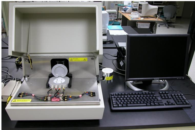
Fig. 27 Equipment of Hall effect measurement system
