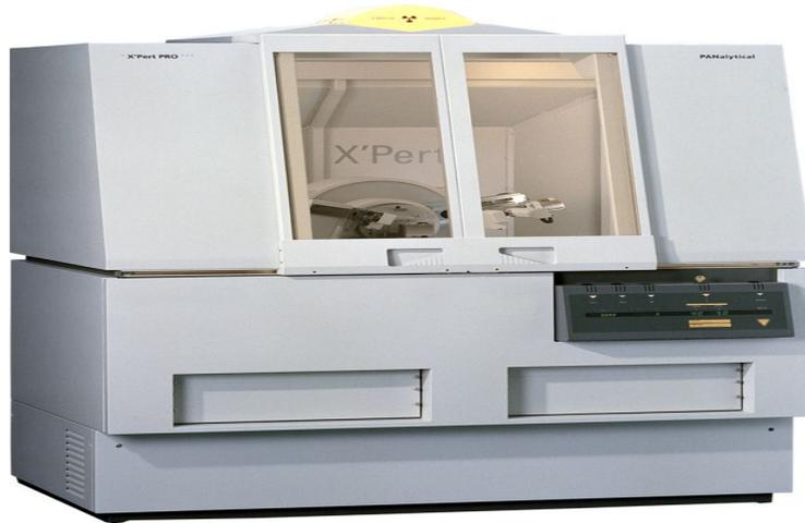
Fig. 23 Equipment of X-ray diffractometer (XRD)
