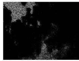
Fig. 68 EDX analysis and element mapping on PTFE and 2.0 g of CNT powder hot-pressed Al sample
