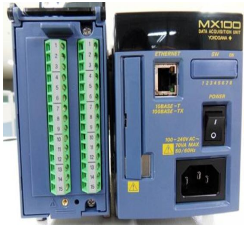
Fig. 4.7 Photograph of data acquisition system
