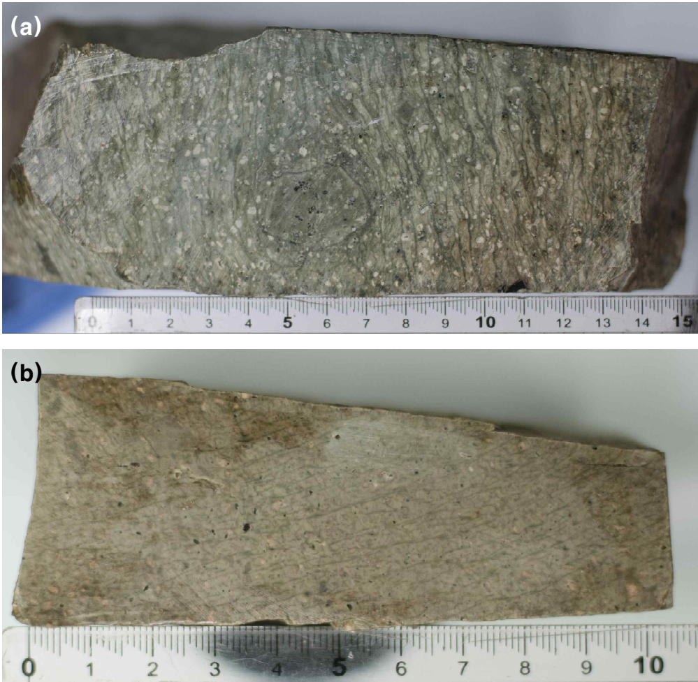
Fig. 28. Photographs of welded tuff on the Goheung area. (a): GH-04, (b)GH-06
