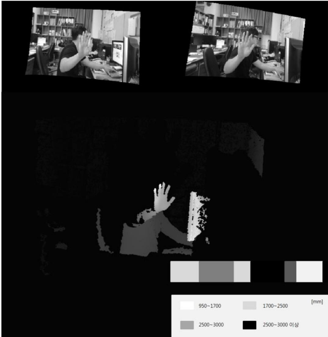
Fig. 4-14 Image fusion and depth map generation
