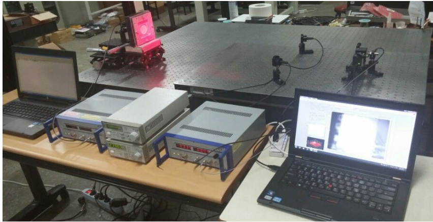
Fig. 4-2 Measurement out of plane deformation using Shearing interferometer
