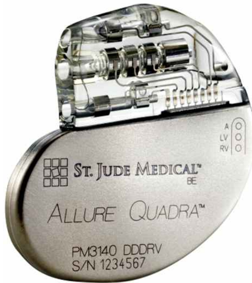
Figure 2.4. Pacemaker applying St Jude’s early wireless power transmission technology.
