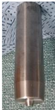
Fig. 3-5 Shape and CAD drawing of FSW tool
