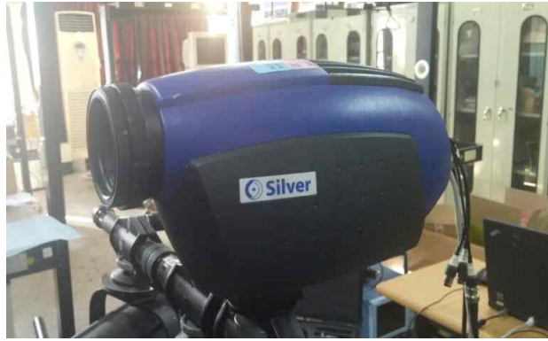
Fig. 3-9 Infrared thermography system
