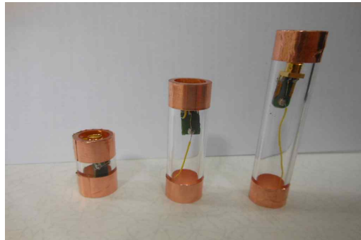
Figure 4-5. Architecture of capsular electrode which located on IMDs
