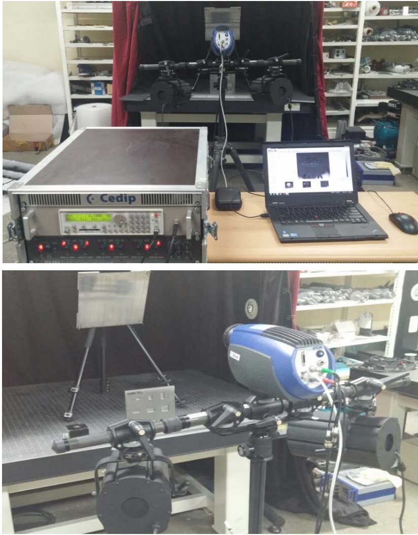
Fig. 3-6 Infrared Thermography system(IRT)
