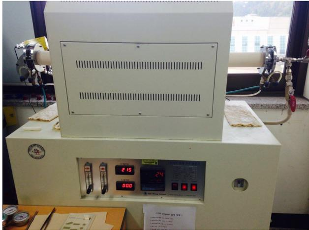
Figure.6 Thermal Chemical Vapor Deposition system used in this study.
