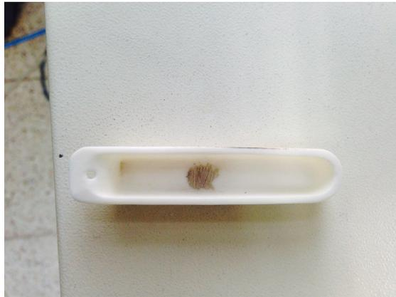
Figure.7 Chemical Vapor Deposition system used ITO powder in this alumina boat.
