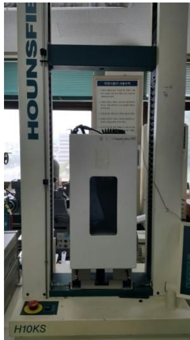
Fig..3.3. tensile composition testing machine and temperature chamber.
