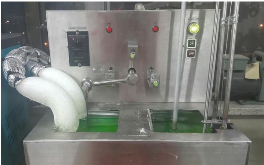
Fig. 3.2 Apparatur for thermal cycling of Ti-Ni alloy wire.
