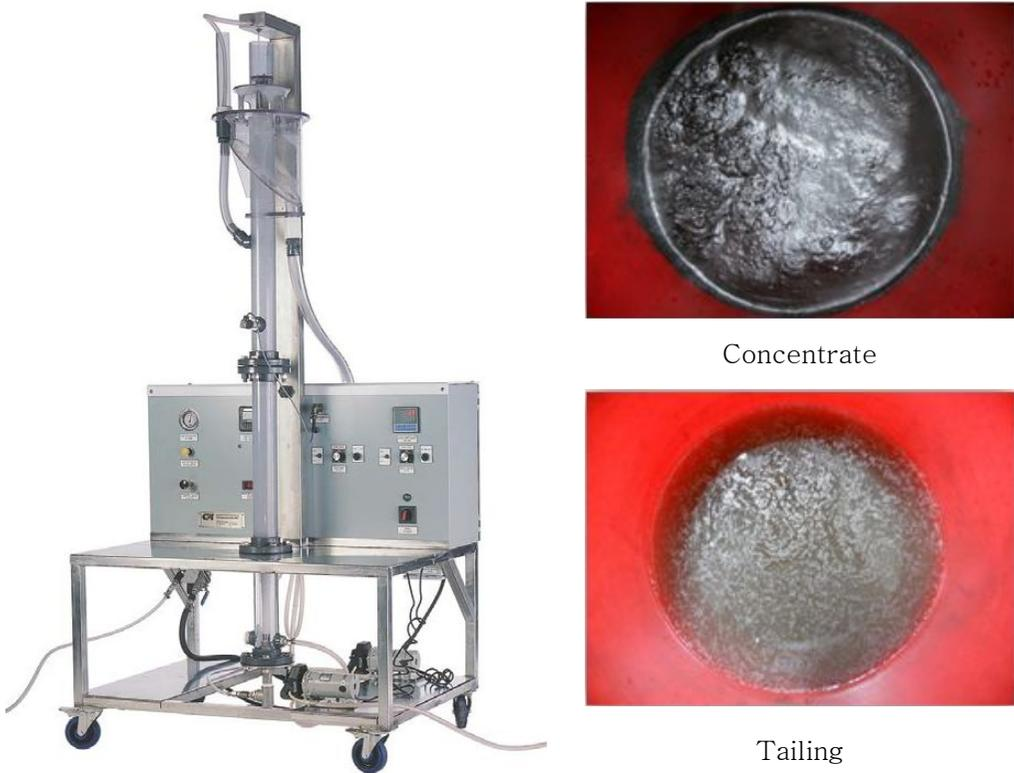
Fig. 3-4. CPT column flotator & concentrate and tailing pictures.
