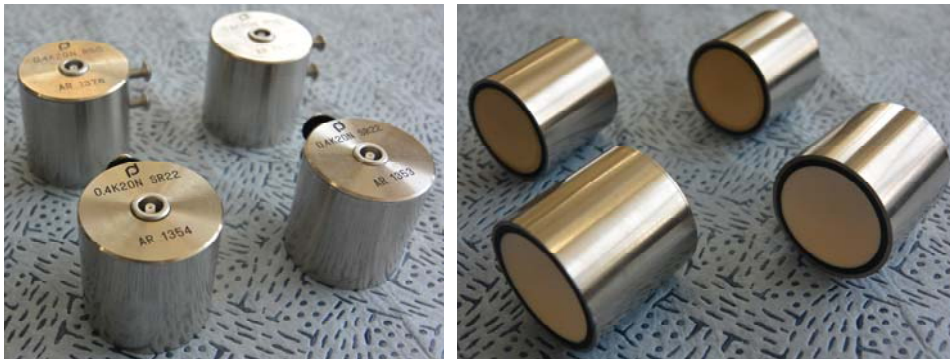
(a) Point focusing type air probe(0.4K20N S50 & S22)
