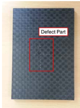
Fig.3-1 Specimens of CFRP
