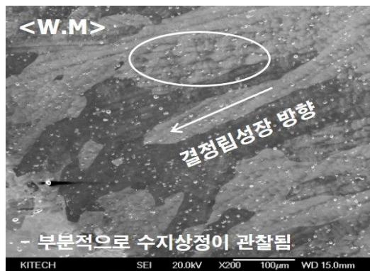
Fig. 3.20 SEM observation in weld metal
