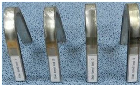
Fig. 3.17 High Mn steel specimen after bending test (19mm)
