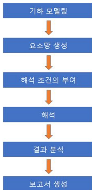
Figure 6.1 Processing flow chart of Soilworks program
