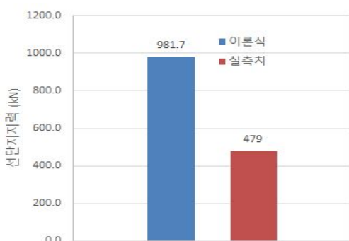
Figure 5.3 End-bearing capacity between theory and fact(Test pile #4)
