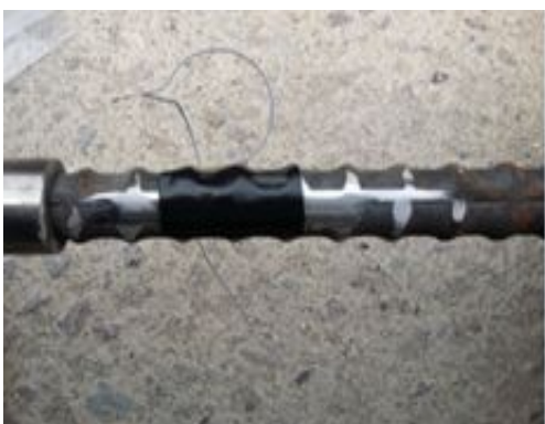
Figure 3.12 The primary waterproofing and wiring
