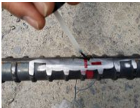
Figure 3.11 Waterproof coating of sensor
