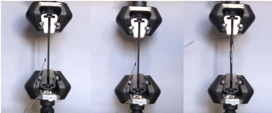
Fig. 36 A Process of Tensile Test  $[0_4/+45_6/-45_6/90_4]_s$
