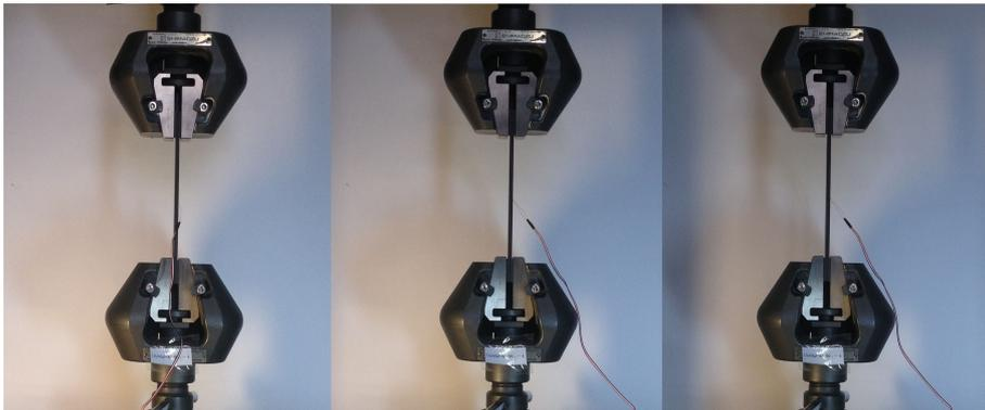
Fig. 34 A Process of Tensile Test  $[0_2/+45_8/-45_8/90_2]_s$
