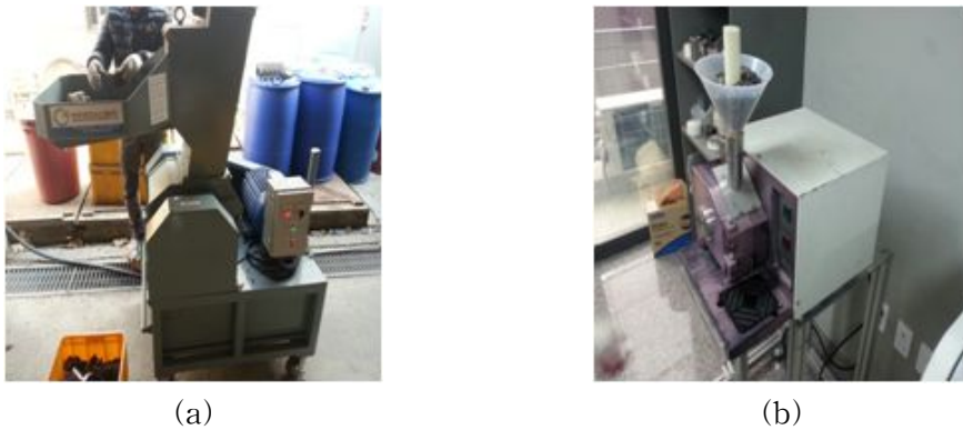
Fig. 3-2. (a)High-speed disintegrator and (b)Cutting mill used in this study
