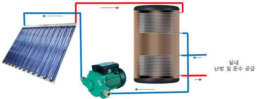
Fig. 6 Solar collector and storage tank system
