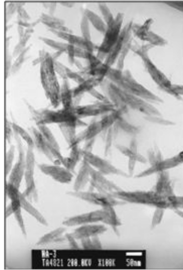
Fig. 4. TEM image of HA nanoparticles.
