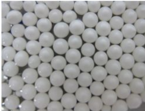
Fig. 2. HA-coated alginate beads.
