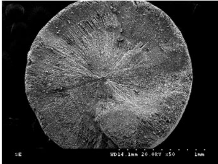
Fig. 6. Cross section of HA showing a solid internal structure.
