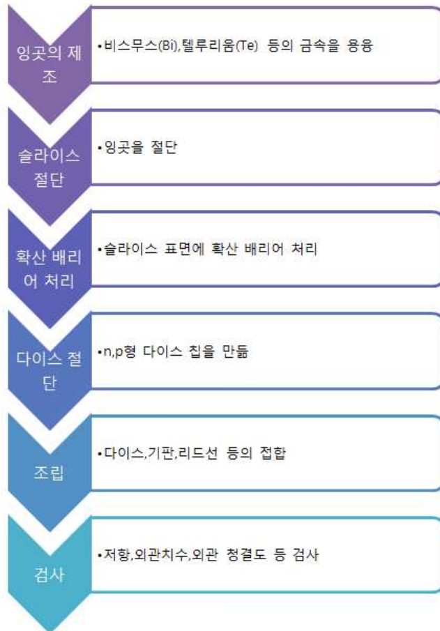
Fig.2-7 The production process of thermoelectric module
