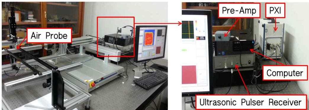
Fig.2-12 Auto image scanning equipment
