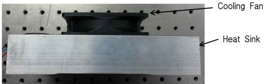
Fig.4-2 Photograph of cooling fan and heat sink Assy
