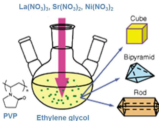
Fig. 4. Process of polyol method
