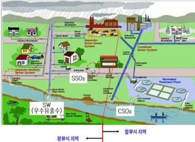
Fig. 1. A schematic diagram representation of the outflow water caused by non-point pollution sources.
