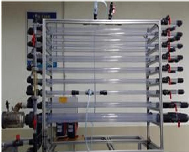
Fig. 6. Photograph of plug flow reactor used in experiments.
