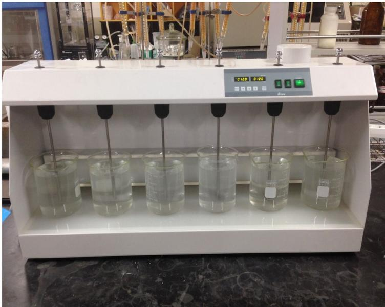
Fig. 5. Photograph of the jar tester used in experiments.
