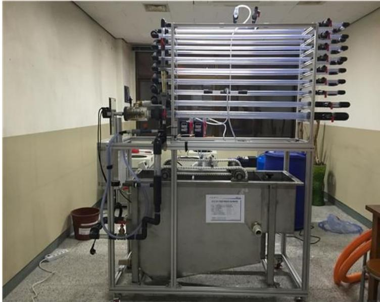
Fig. 7. Photograph of rapid coagulation system used in experiments.
