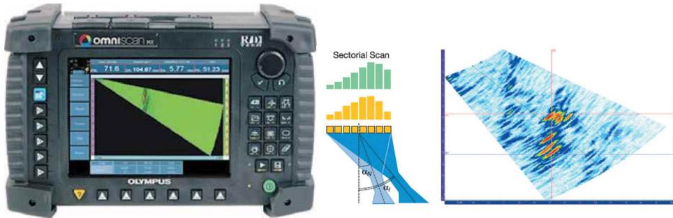
Fig.1-6 PAUT system and flaw detecting image
