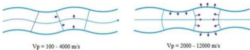
Fig.2-6 Asymmetric mode and symmetric mode of lamb wave
