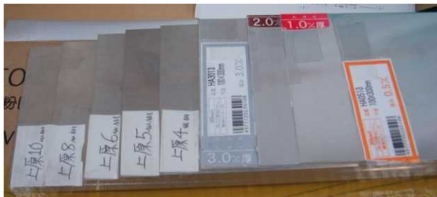
Fig.3-3 Specimens of aluminum(Defect and no defect)
