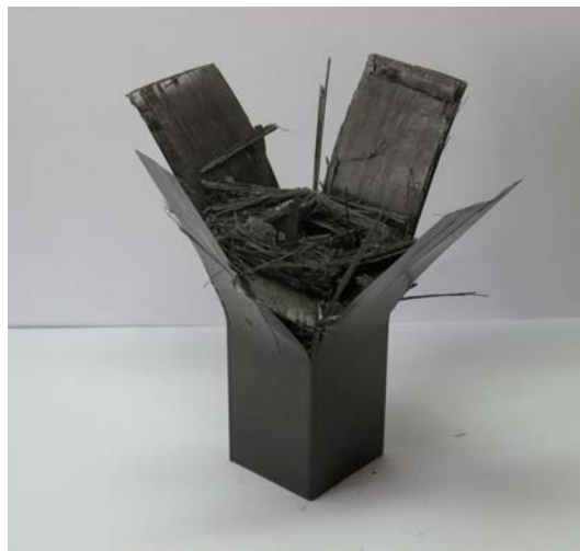
Photo. 5 Shape of collapse CFRP square shaped section member, [90^\circ / 0^\circ]_4 (Impact Energy 372.4J)
