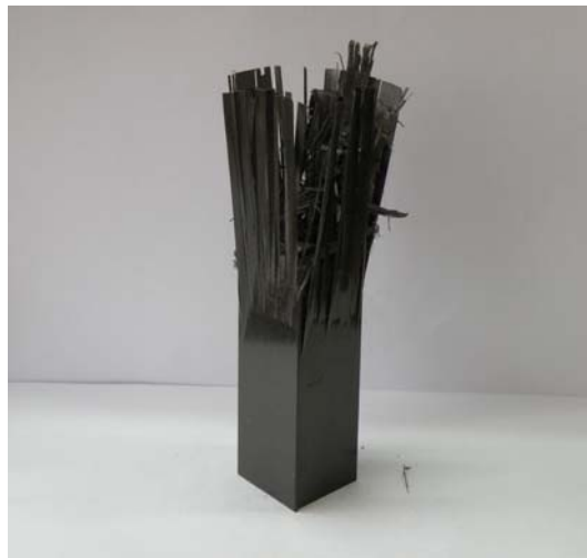
Photo. 3 Shape of collapsed CFRP square shaped section member, [-15^\circ / +15^\circ]_4 ( Impact Energy 372.4J)
