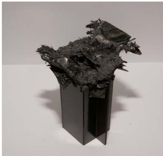
Photo. 10 Shape of collapsed CFRP double hat shaped section member, [+45^\circ / -45^\circ ]_4 (Impact energy 611J)
