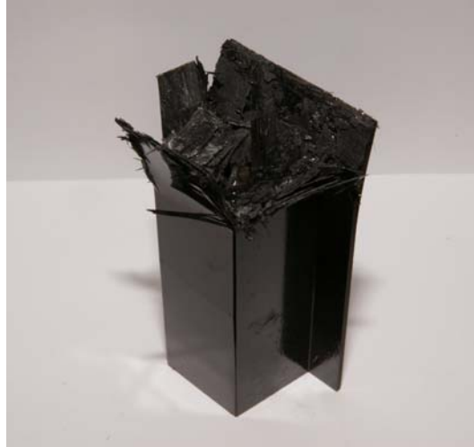
Photo. 15 Shape of collapsed CFRP single hat shaped section member, [+15^\circ / -15^\circ ]_4 (Impact Energy 419J)
