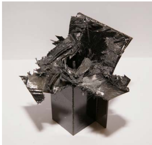
Photo. 7 Shape of collapsed CFRP single hat shaped section member, [+45^\circ / -45^\circ ]_4 (Impact energy 419J)
