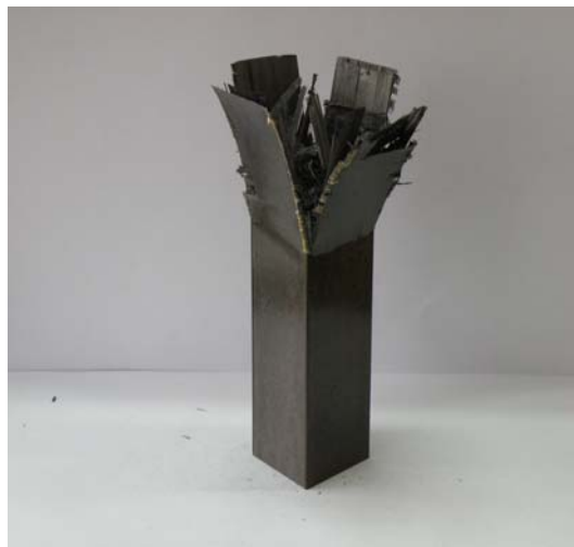
Photo. 4 Shape of collapsed CFRP square shaped section member, [-45^\circ /+45^\circ ]_4 ( Impact Energy 372.4J)
