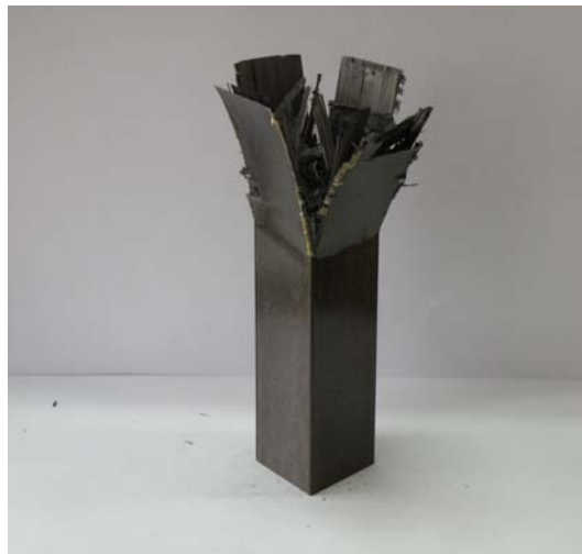
Photo. 13 Shape of collapsed CFRP square shaped section member, [-45^\circ / +45^\circ]_4 (Impact Energy 372.4J)
