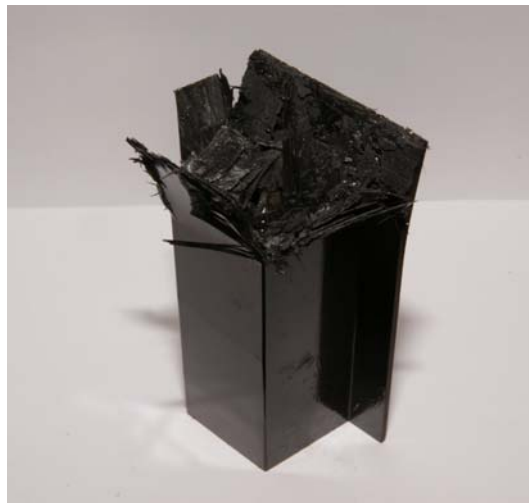
Photo. 6 Shape of collapsed CFRP single hat shaped section member, [+15^\circ / -15^\circ ]_4 (Impact energy 419J)
