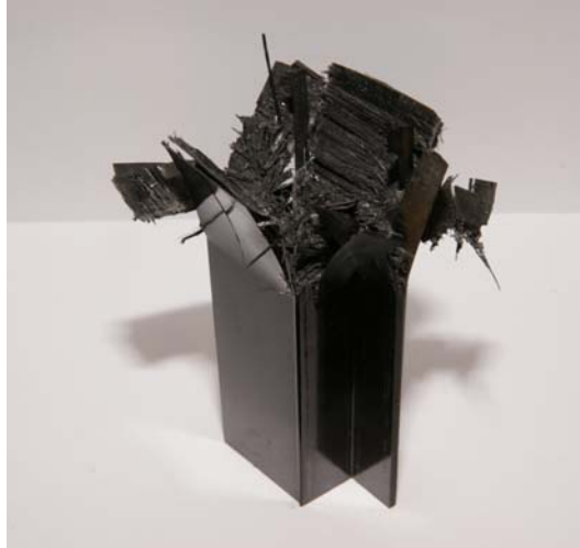
Photo. 20 Shape of collapsed CFRP double hat shaped section member, [90° /0° ] 4 (Impact energy 611J)
