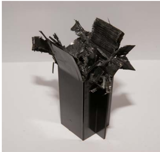
Photo. 11 Shape of collapsed CFRP double hat shaped section member, [90^\circ / 0^\circ]_4 (Impact energy 611J)
