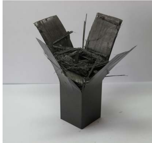
Photo. 14 Shape of collapsed CFRP square shaped section member, [90^\circ / 0^\circ]_4 (Impact Energy 372.4J)
