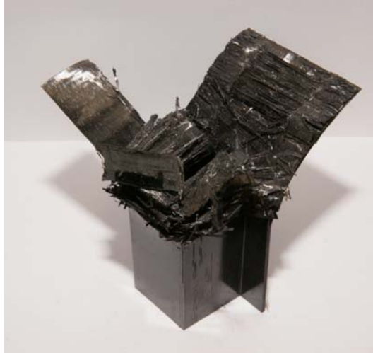
Photo. 17 Shape of collapsed CFRP single hat shaped section member, [90° /0° ] 4 (Impact energy 419J)
