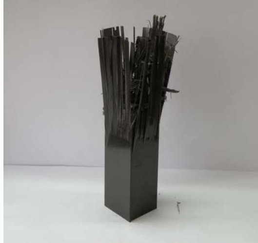
Photo. 12 Shape of collapsed CFRP square shaped section member, [-15^\circ / +15^\circ]_4 (Impact Energy 372.4J)
