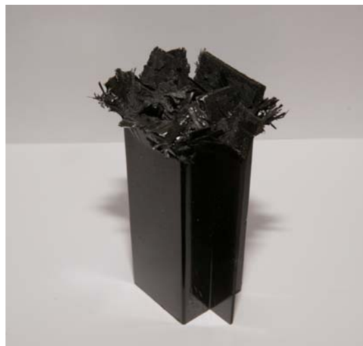
Photo. 9 Shape of collapsed CFRP double hat shaped section member, [+15^\circ / -15^\circ ]_4 (Impact energy 611J)
