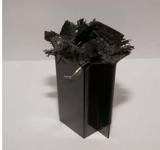
Photo. 18 Shape of collapsed CFRP double hat shaped section member, [+15° /-15° ] 4 (Impact energy 611J)
