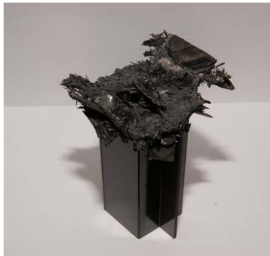
Photo. 19 Shape of collapsed CFRP double hat shaped section member, [+45° /-45° ] 4 (Impact energy 611J)
