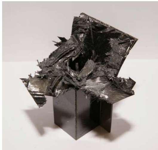
Photo. 16 Shape of collapsed CFRP single hat shaped section member, [+45^\circ / -45^\circ ]_4 (Impact energy 419J)
