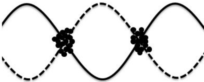
(c) Particles forming clumps in the nodal point
