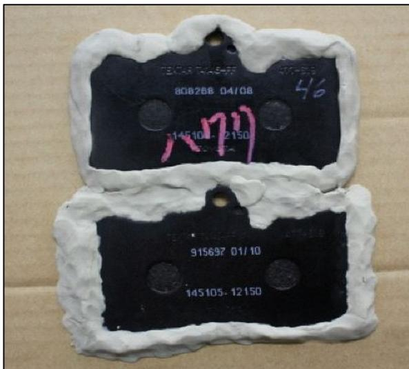
(a)Compensated specimen brake pad A, B
