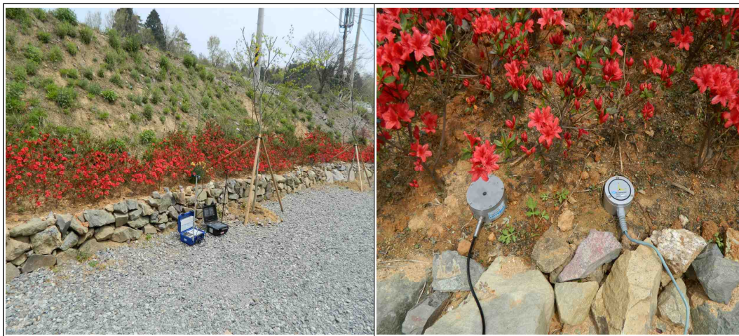
Figure 5.4 View of measuring blasting vibration in soil ground
