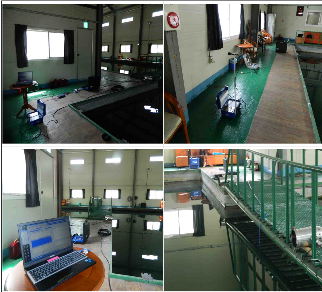
Figure 5.5 View of measuring blasting vibration and underwater noise in fishing water tank
