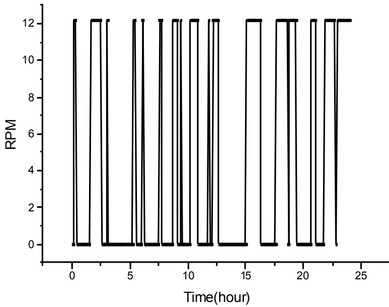
Fig. 3-17 Operation pump for on-off control dilution rate in 1.0\text{day}^{-1}
