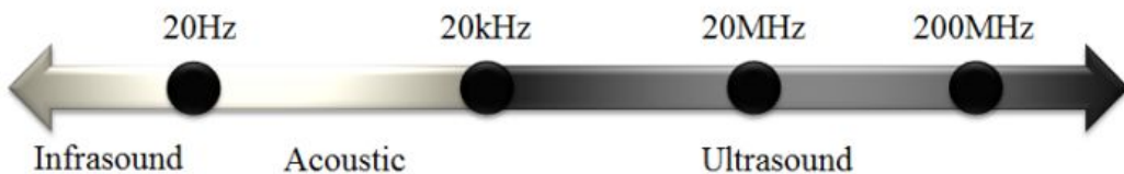
Fig. 2-1 Classification of the sound waves according to the frequency
