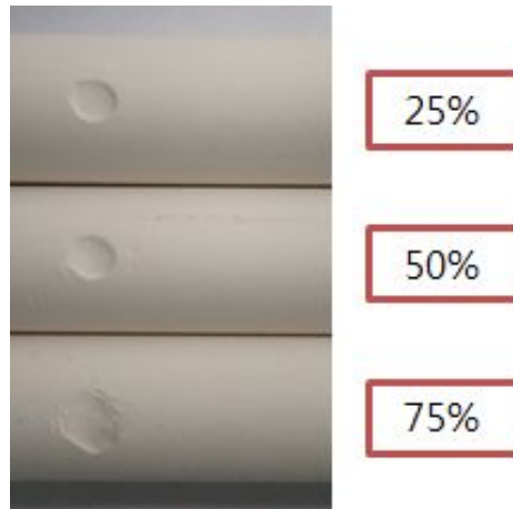
Fig. 5-1 Hole shape of CaCO 3 according to on/off ratio
