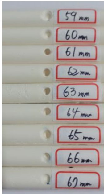
Fig. 4-6 Hole shape according to focal distance(couplant: water)
