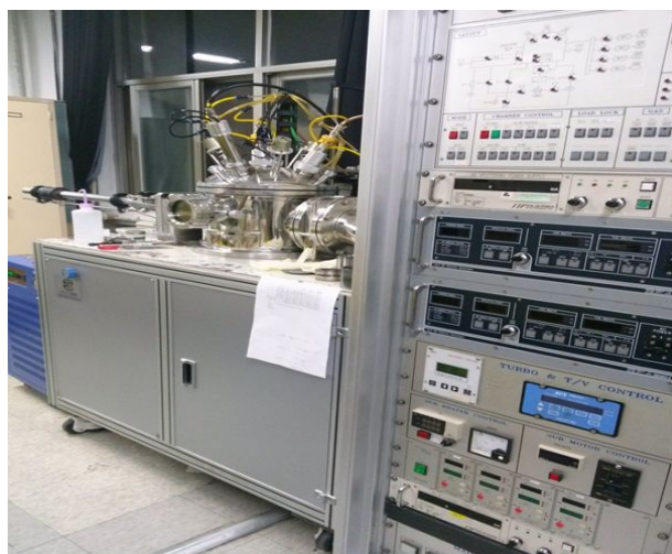
Fig. 3 RF magnetron sputtering equipment (I.D.T. ENG)
