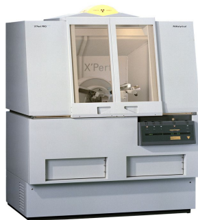
Fig. 6 XRD equipment (Philips X'pert-PRO-MRD XRD)
