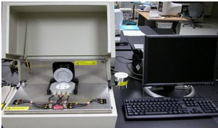
Fig. 8 Hall effect measurement system equipment (Accent Optical Technologies. HL5500PC)
