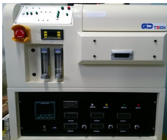
Fig. 4 Rapid thermal annealing equipment (GD Tech)
