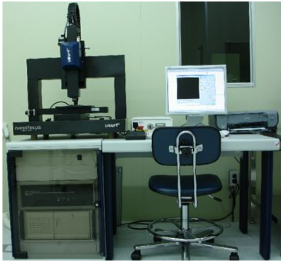
Fig. 3-6 Surface Profiler System
