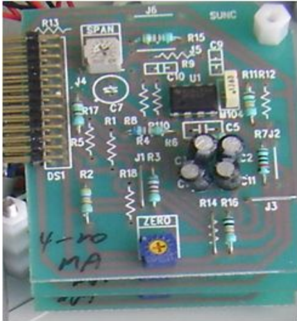
Fig. 3-8 PCB & circuit of pressure sensor
