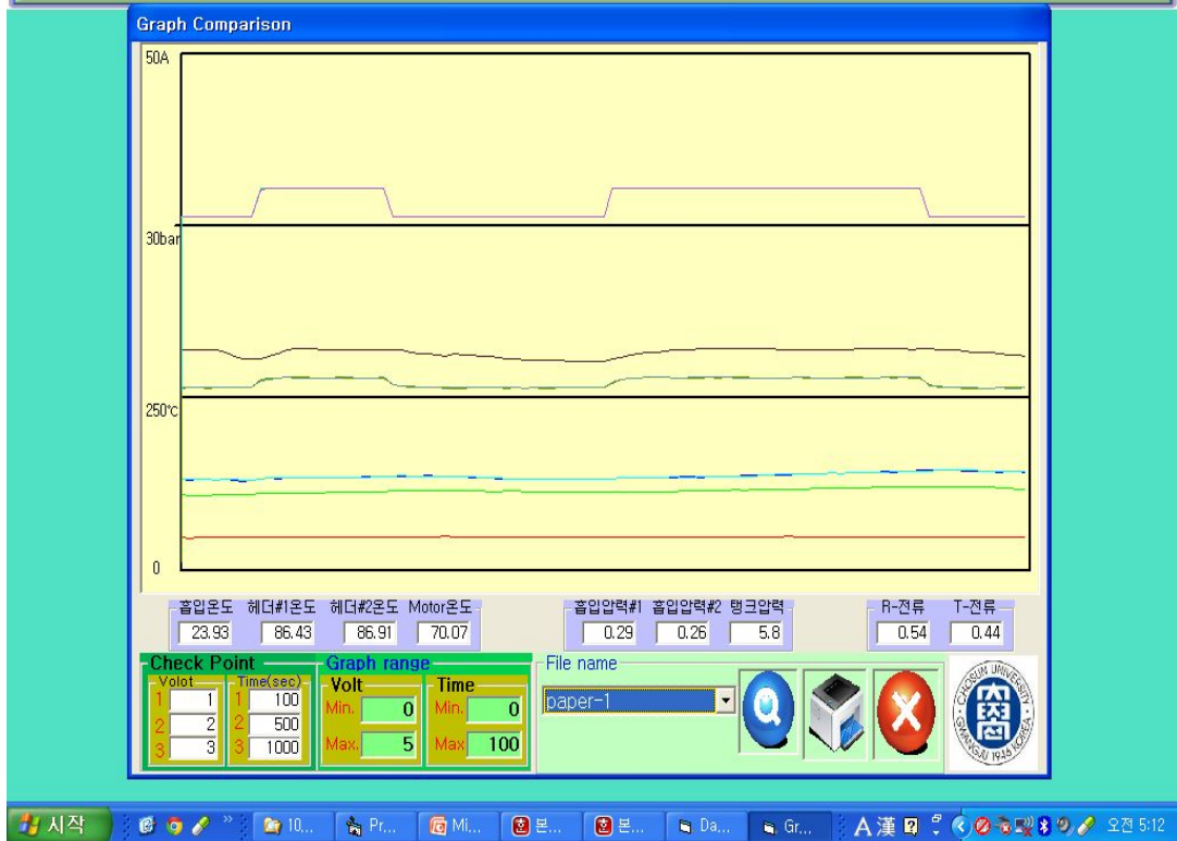
Fig. 3-17 PC monitoring for sensor signal of air-compressor
