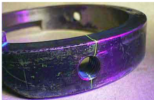
Fig. 1-6 Magnetic particle wet fluorescent indication of cracks in a fastener hole [19].
