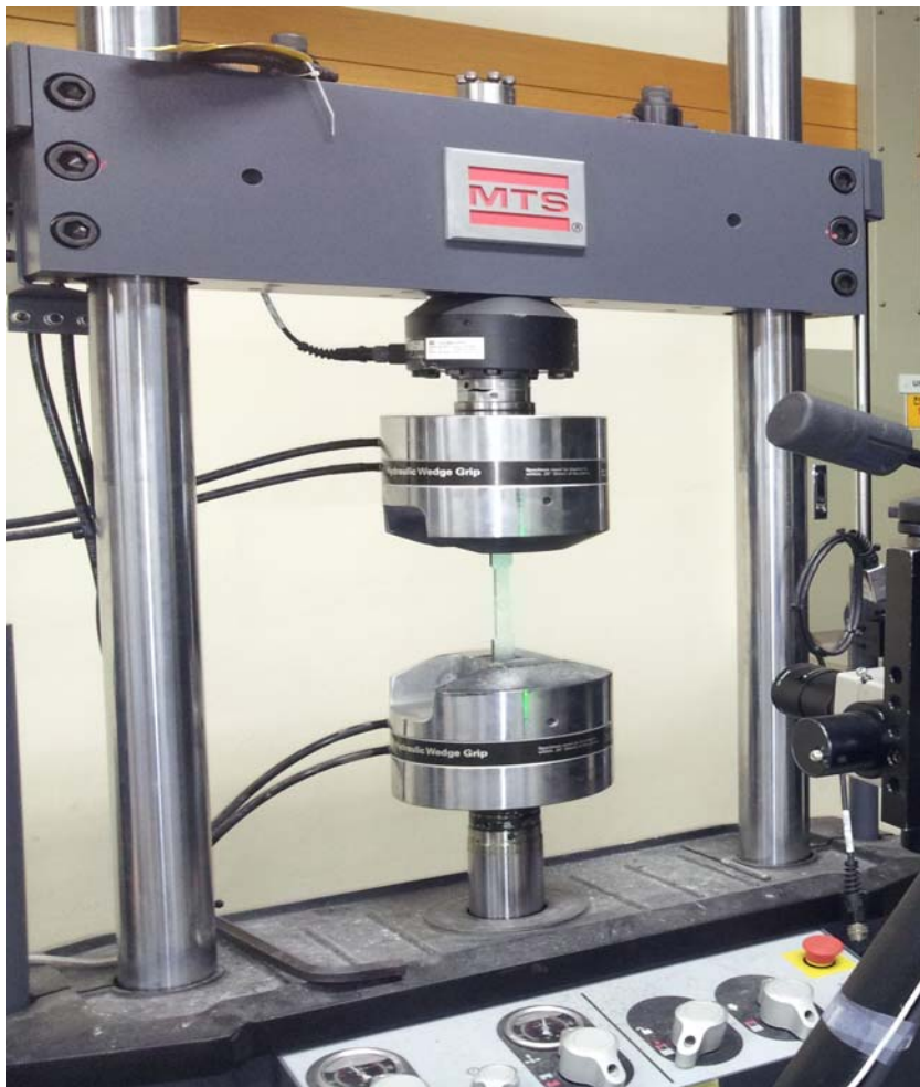
Fig. 3-3 MTS system for tensile loading
