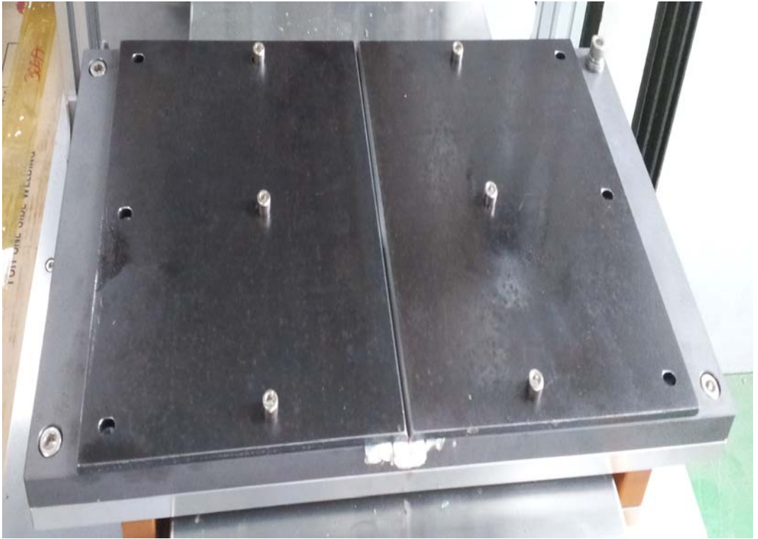
Fig. 3-7 Fabricated welding jig
