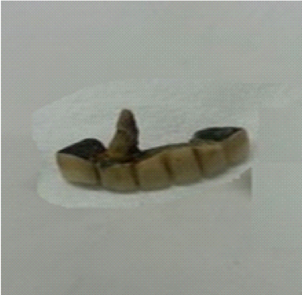
Fig 3-3. A picture of Ni-Cr alloy composite dental prosthesis extracted from a dental patient after about four years usage.
