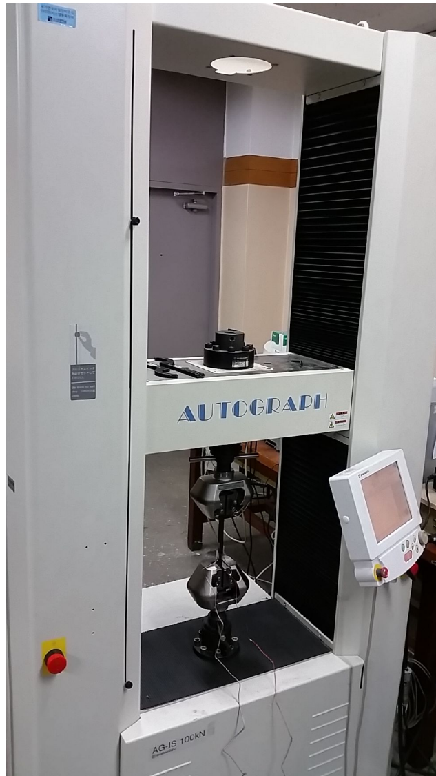
Photo. 3 Universal Testing Machine (Tensile Testing)
