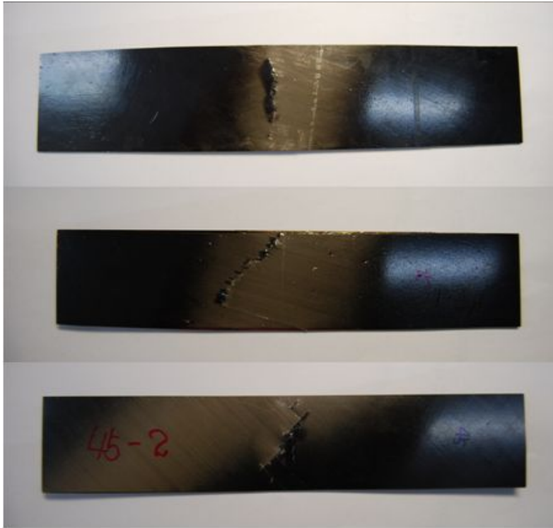
Photo. 17 Test specimens of Bending Fracture
