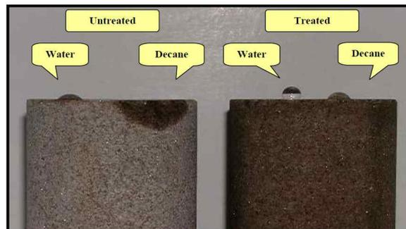
(b) Contact angle for untreated and treated reservoir cores
