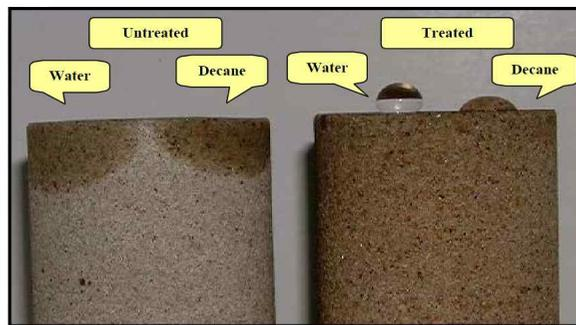
(a) Contact angle for untreated and treated Berea
