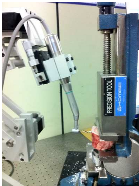
Fig. 4-7 Drilling into the cow bone using ARDIS
